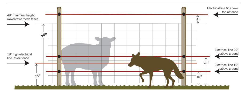
The fence has a total of four electrical lines.
